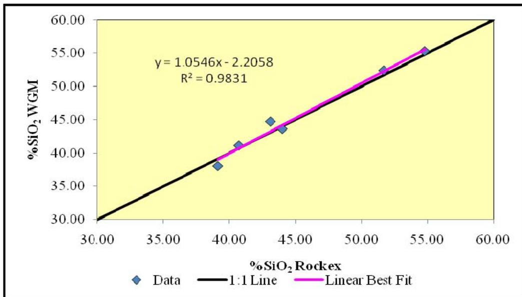
Figure 34. %SiO<sub>2</sub> for WGM Independent Samples vs. Rockex Original
