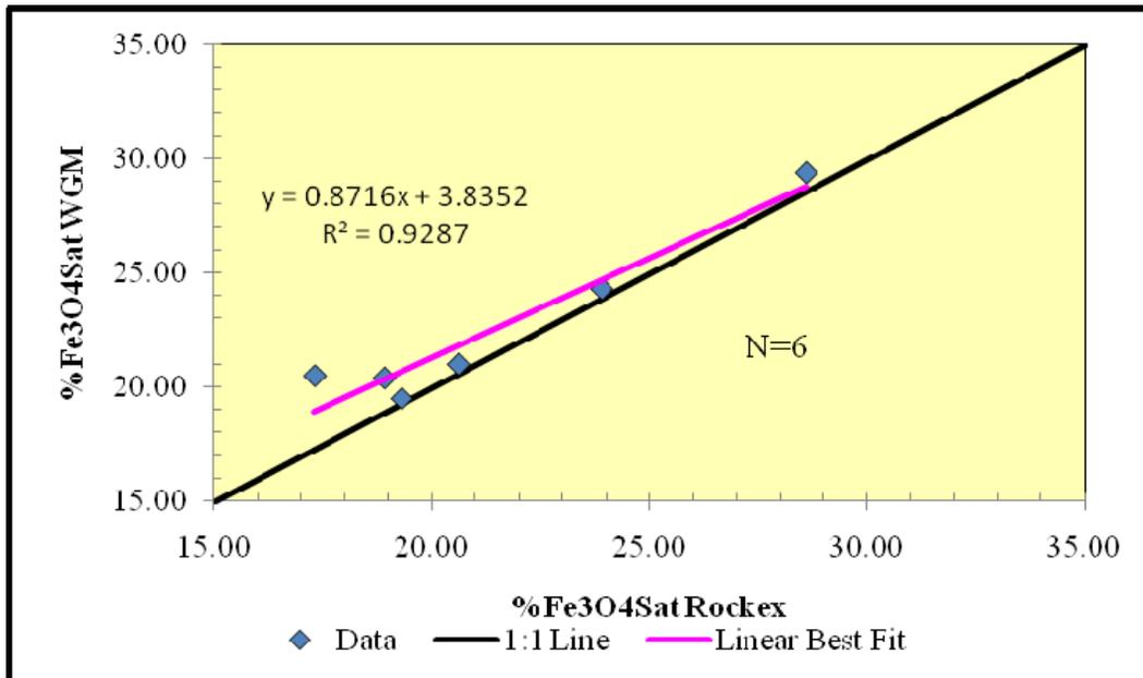
Figure 32. %Fe<sub>3</sub>O<sub>4</sub> Satmagan for WGM Independent Samples vs. Rockex Original
